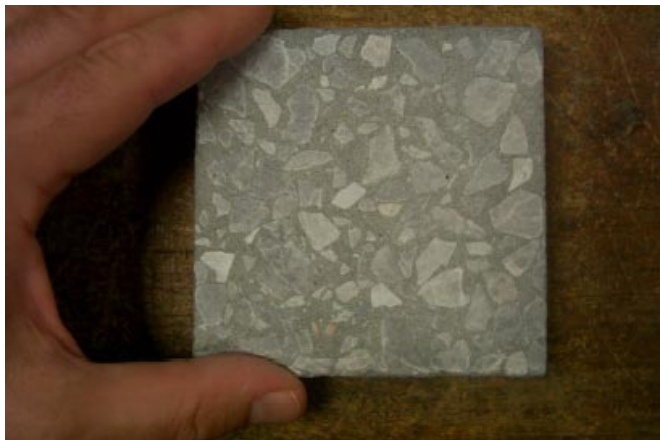
A typical EMR specimen from the Port. Note the tight spacing of the coarse aggregate. Even with 51% coarse aggregate by volume (most concrete today falls within the range of 38 to 44%), these mixtures provided highly cohesive concrete with slump values generally more than 10 cm, that were pumped, conveyed or bucketed into position. Photo courtesy of the University of Wales, Swansea; EMR specimen provided by Delmon Ready Mixed Concrete Products of Bahrain.
