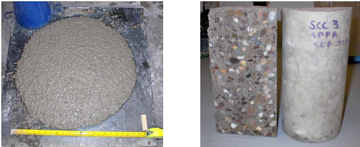
Figure 5. Mix SPFA1 following a slump flow test and the aggregate distribution in a hardened sample
